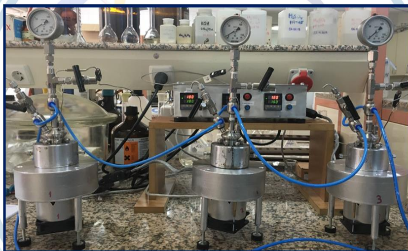
Figure 1. Batch, stirred and temperature-controlled reactor system
